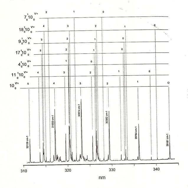
Fig. 1. Laser excitation fluorescence spectrum of the B  $^2A'$  - X  $^2A''$  system of the ethoxy radical. The time delay between the excimer laser and the dye laser was 8  $\mu$ s.
