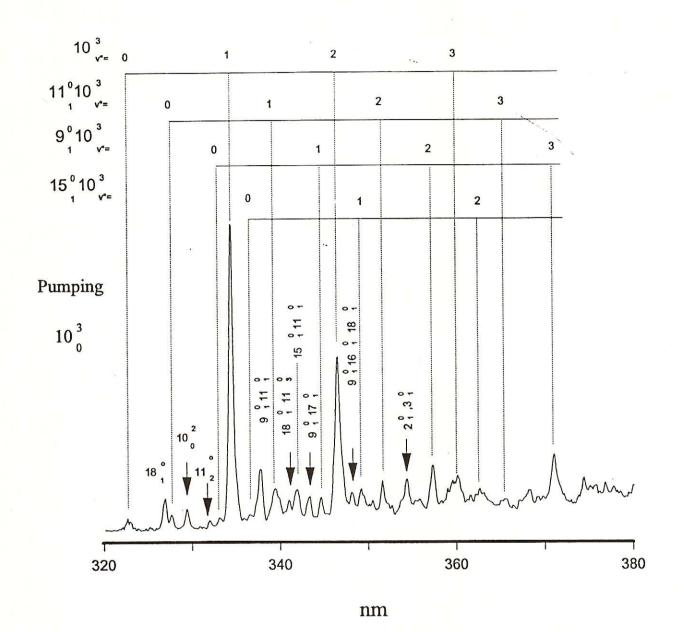
Fig. 2. The dispersed spectrum of the B-X  $10_0^3$  band of the ethoxy radical. The frequency of the pump laser was 30972 cm<sup>-1</sup> and the time delay between the excimer and dye lasers was 5  $\mu$ s.
